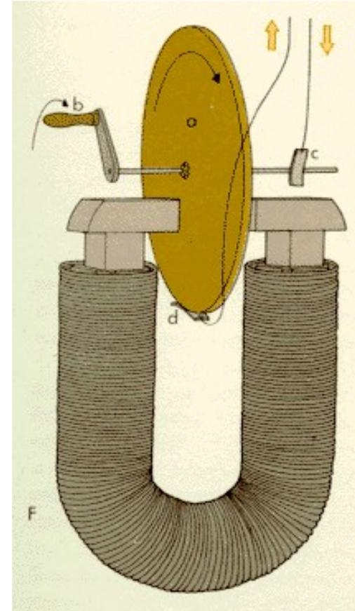
*Faraday's disk dynamo* - for producing continuous (pure) dc voltage. This was the world's first electrical generator.
