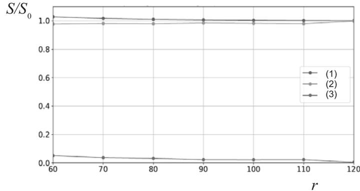
**Figure 2.** Electromagnetic energy flux from the region of closed (lower curve) and open (middle curve) magnetic field lines. The upper curve corresponds to the total energy loss. The radius of the neutron star (40 cells) is 10 times smaller than the radius of the light cylinder.
