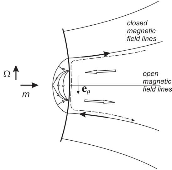
**Figure 1.** The structure of the volume (contour arrows), separatrix (fat arrows) and surface (thin arrows) currents near the polar cap of the orthogonal rotator. The additional separatrix current is shown by a dashed curve.
